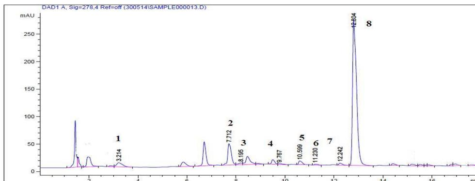
Figure 1: HPLC chromatogram of polyphenol-rich extract of *Gomphus floccosus* (*GfPre*) (MP: mobile phase, peaks: 1: gallic acid, 2: caffeic acid, 3: vanillic acid, 4: ferulic acid, 5: myricetin, 6: salicylic acid, 7: cinnamic acid, 8: pyrogallol)
